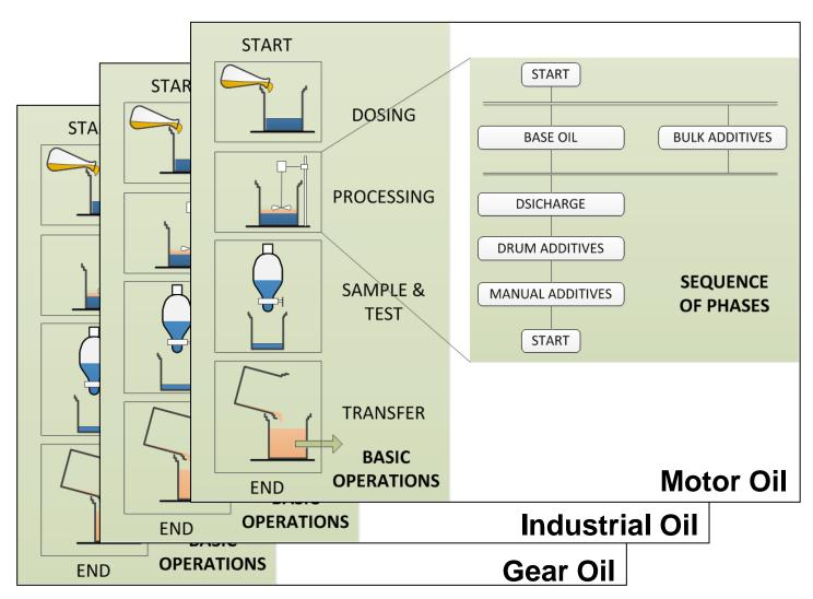
The lubricant plants are mostly designed as 'multiple product / multiple line plants'. High flexibility in the production can only be reached by
